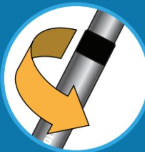
4 Before detaching the poles, release all twist-lock fasteners entirely. Then with one pull separate the segments from each other.
