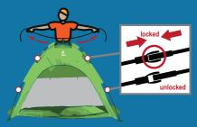
All pole joints (see red marking) have to be in the "locked"-position (see detail view).
