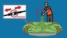
**Caution:** Before continuing with step 3 the pole joints have to be unlocked (see "unlocked"-position). Just open - as shown in the detail view - on all four poles the joint parts.
